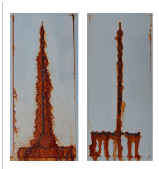
Figure 5: Protective effect of polymeric corrosion inhibitors in a polyurethane coating on steel
